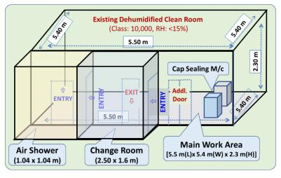
(2000 CFM, designed for <15%RH, make: Bry-air); and Clean room panel with insulated Ducting systems, ADS (air distribution system), VCD (volume control dampers), Fire dampers; ERAR (external return air raisers), Anti-static flooring, Electrical panel with wiring for lights/machines and separate Plant room, where all the machines are housed.
