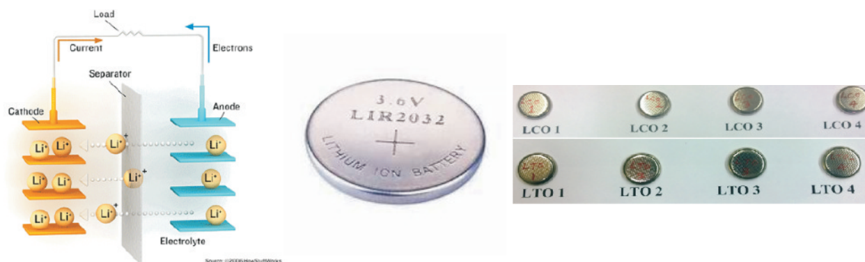
Fig.1.1 Schematic of the mechanism of Li-ion batteries, a typical button/coin (2032 type) cell and prototype cells fabricated at C-MET
