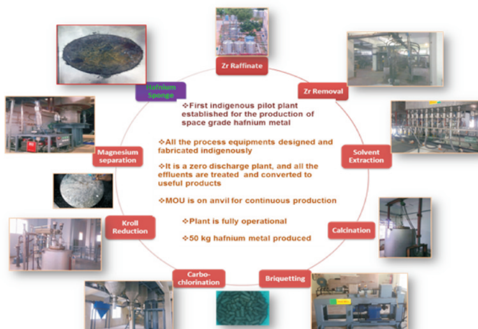
Fig. 3.1 Major process steps in preparation of hafnium sponge
