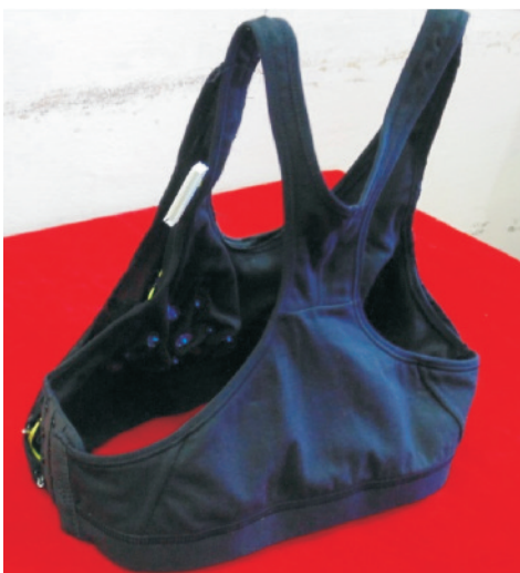
Fig. 10.1 The wearable device developed by C-MET for screening of breast cancer.
