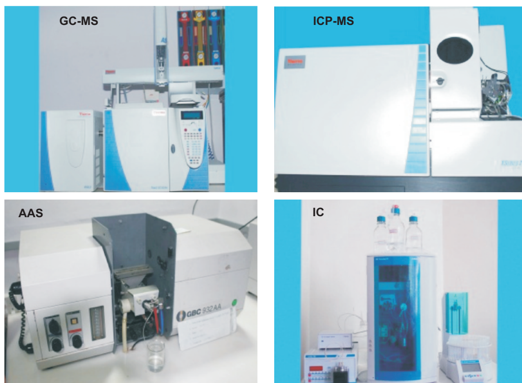
Fig.6.1 Important analytical instruments used for RoHS testing
