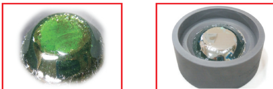
Fig. 4.1 Two inch diameter 6H SiC (L) and 4H SiC (R) single crystals
