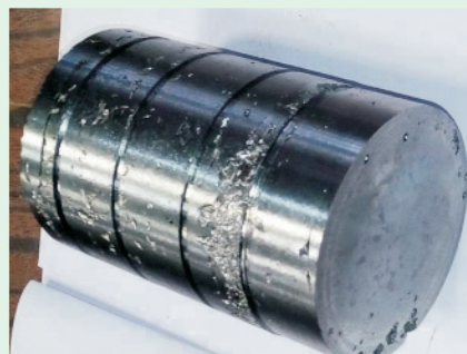
E-beam refined Hafnium (Hf) from Hf sponge
