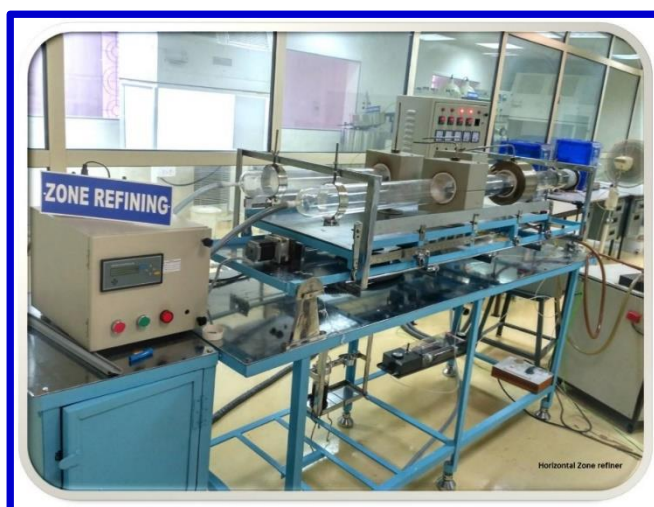
Figure 10. Resistive zone refining system and purified tellurium and cadmium
