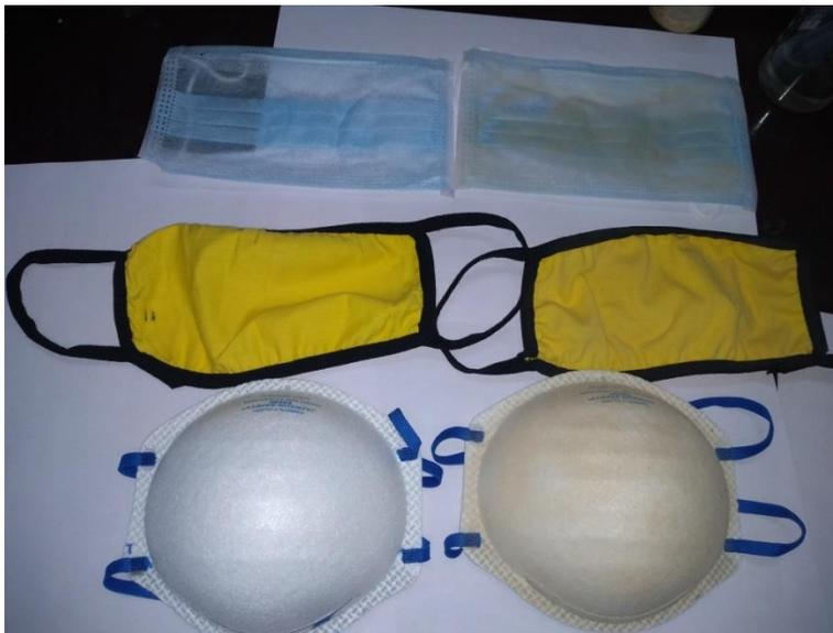
Photo shows the three types of mask, left side are without coating and right side are nanoparticle coated mask.
