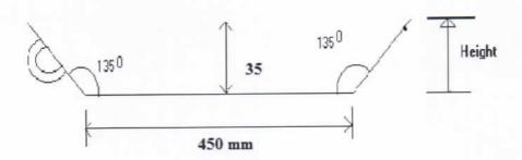
Quartz Boat: Longitudinal section; Dimensions: a) Length- 450 mm, b) Height -35.0 mm
